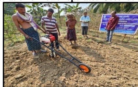
Demonstration of Engine operated post hole digger for establishment of trellis in Pointedgourd
